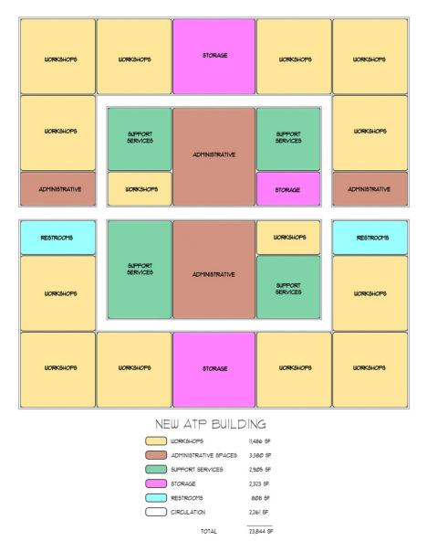
Figure 23: ATP Potential Improvements – ATP Functions - Option 2 – New ATP Building
