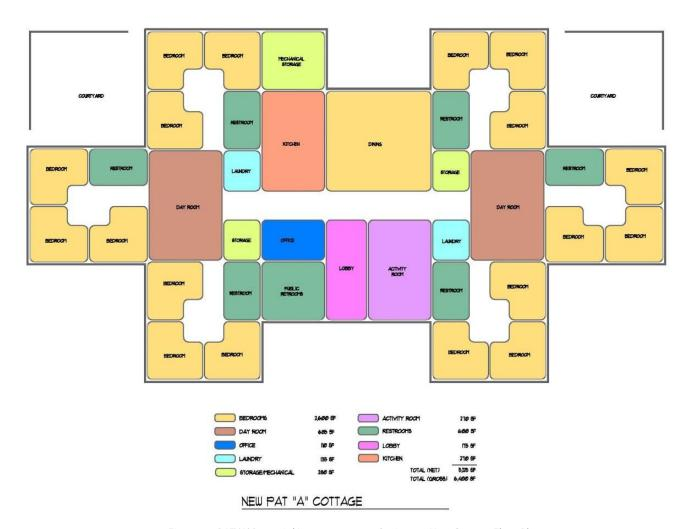
Figure 26: PAT 'A' Potential Improvements – Option 1 – New Cottage Floor Plan
