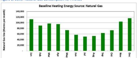
Figure 2. Boiler Natural Gas Consumption for Fircrest
