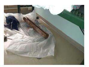
Birch Bldg. Corroded Waste Piping and Piece of Floor Slab
