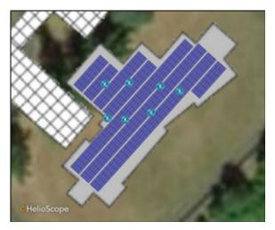
Figure 1: 186 kW Solar PV Array Concept for Maple Lane Site
