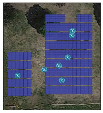
Figure 13: 186.3 kW Rooftop & Ground-mount Solar PV Array
