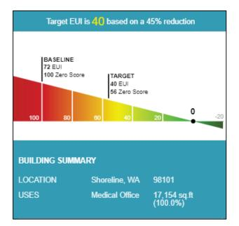
Figure 3: Energy Use Intensity (EUI) Baseline and Target
