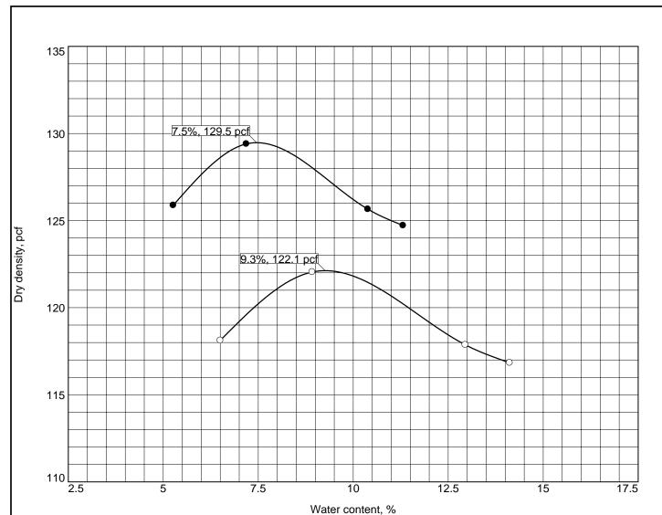
Test specification: ASTM D 1557-91 Procedure C Modified ASTM D4718-15 Oversize Corr. Applied to Each Test Point
